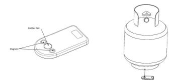
Installing SmartSense Sensors
