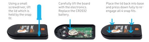
Replacing SmartSense Sensor Batteries
