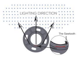
The installation direction of the base directly determines the direction of the lighting, The light will shine in the direction opposite to the sawtooth
