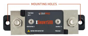
Use two appropriately sized screws with a screw head no larger than 12mm to secure the XShunt500 to a solid surface. The type of screw required will depend on the surface material you are mounting the XShunt500 to.
