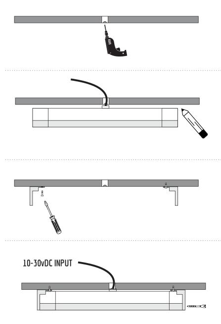
**A**. Drill 18mm hole for cable. This should be drilled in relation to the centre of light position.
