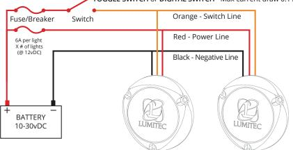
To use the 3-wire system, simply connect the red and black 10-30VDC lines to an appropriately fused power buss with constant power and the Orange wire to a switched +10-30VDC buss referenced to the same ground as the power lines.
