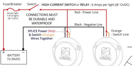
NOTE: The SBX2 can also be wired in a standard two wire installation as well by simply connecting the red and orange wires together and powering via an appropriately rated switched power buss.
