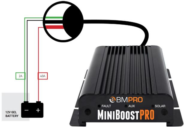
Figure 2: Selecting the 12VGel Battery
