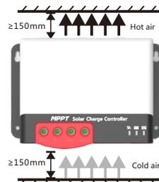
Figure 2.1 Installation and Heat Dissipation
