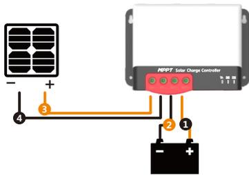
**⚠ Warning: Danger, Electric shock hazards!** We strongly recommend connect a fuse or circuit breaker to the PV array and battery terminals to prevent electric shock hazards during wiring or error operation, and make sure that fuse or circuit breaker is disconnected before wiring.
