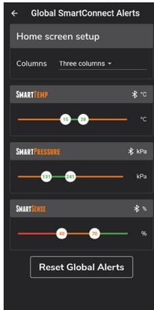
Drag the sliders to set your alarm thresholds for each type of SmartConnect sensor. If a value falls outside the green zone, a notification will display.
