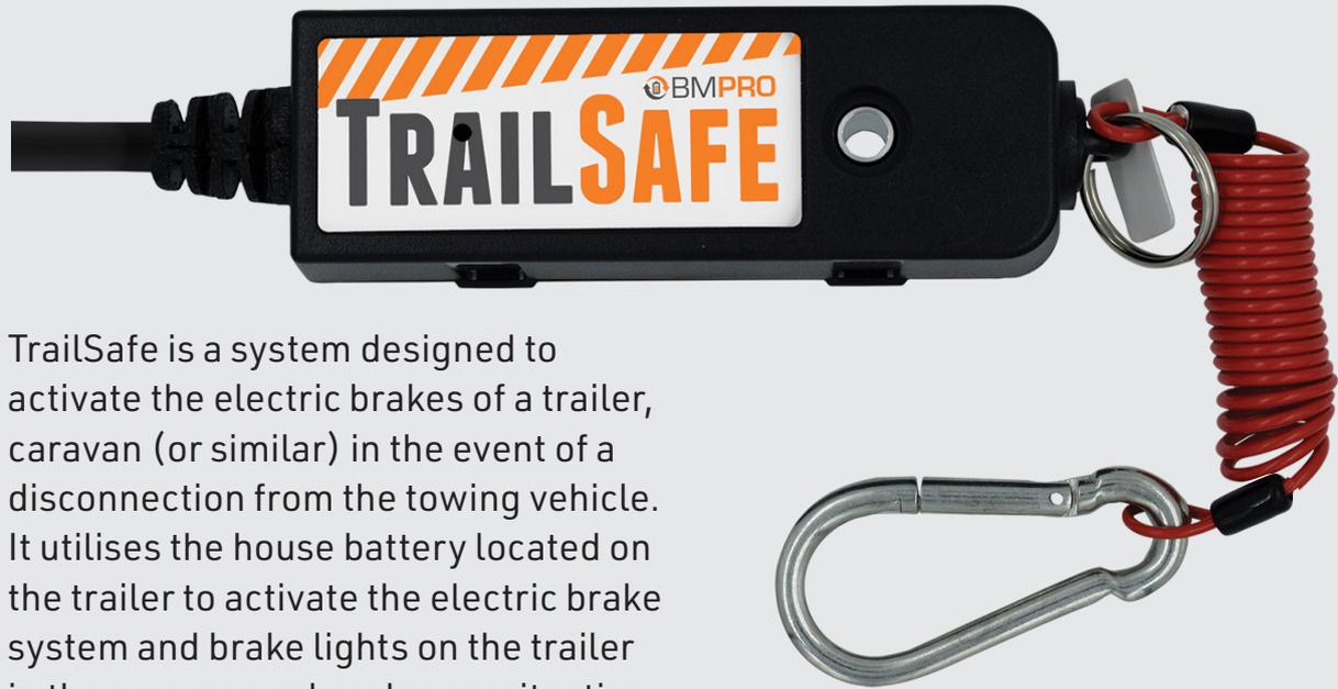
TrailSafe is a system designed to activate the electric brakes of a trailer, caravan (or similar) in the event of a disconnection from the towing vehicle. It utilises the house battery located on the trailer to activate the electric brake system and brake lights on the trailer in the emergency breakaway situation.
