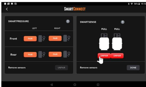
Figure 14: Unpairing the SmartSense gas bottle level sensor
